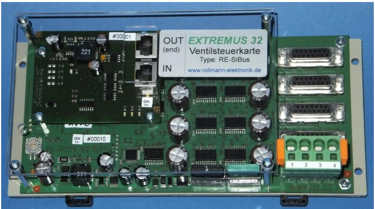
image with RE-SiBus-interface for expansion of Modbus/TCP or other bus interfaces (Profibus, ProfiNET, EtherCAT...)
